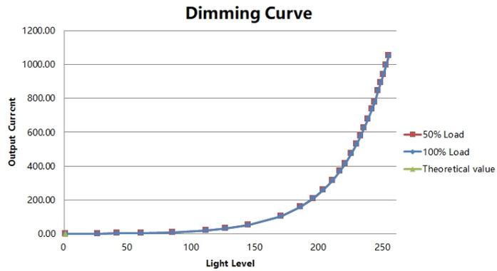
Note: Test data under 1050mA gear
