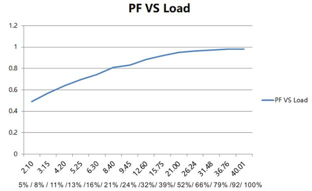
Note: Test data under 1050mA gear
