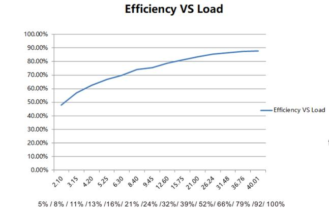
te: Test data under 1050mA gear
