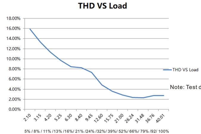
Note: Test data under 1050mA gear
