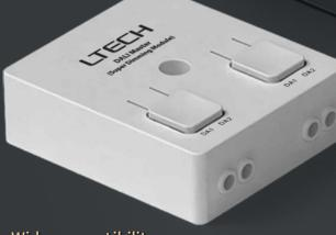
Wide compatibility Support DALI-2 DT6,DT8 Tc, DT8 XY and RGBWAF.Control DIM,CT,RGB,RGBW, RGBCW lights with 1-5 channel Extensive applications Combine Bluetooth products to create local/automated scenes.Control local scenes without the Internet or a gateway. Bind smart switches
